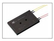
**ACP's** 100 GHz 1 Channel OADM utilizes thin film coating technology and proprietary design of non-flux metal bonding micro optics packaging to achieve optical add and drop at the ITU wavelength. It provides ITU channel center wavelength, low insertion loss, high channel isolation, wide pass band, low temperature sensitivity and epoxy free optical path. It can be used for wavelength add/drop in telecommunication network system. All AC Photonics' products are Telcordia qualification tested.
